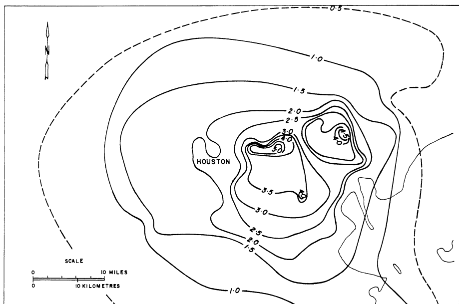
Fig. 1-16b. Subsidence of land surface (in feet) in same area as Figure 1-16a over same period (after Gabrysch, 1967, fig. 19, by courtesy of the Texas Department of Water Resources).
